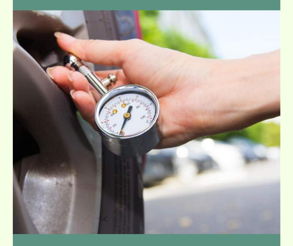
Underinflated tyres generate more friction on the road and this causes higher fuel consumption.
